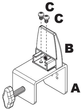
**1** Attach B to A with Screws C
