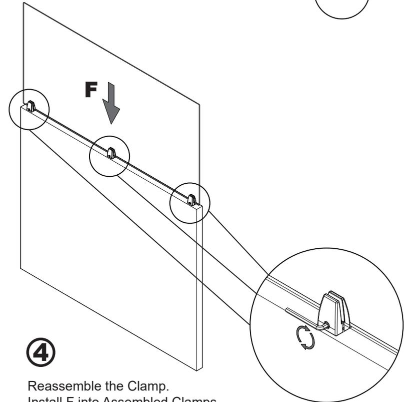
**4** Reassemble the Clamp. Install F into Assembled Clamps. Tighten Clamps.
