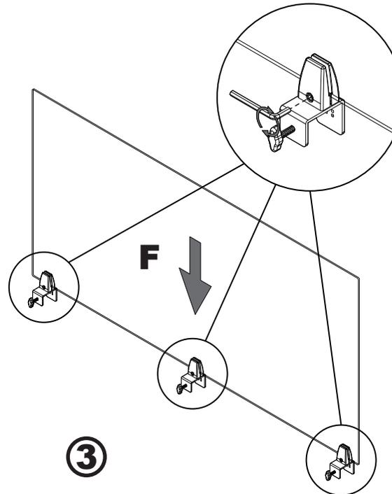
**3** Install F into Assembled Clamps
