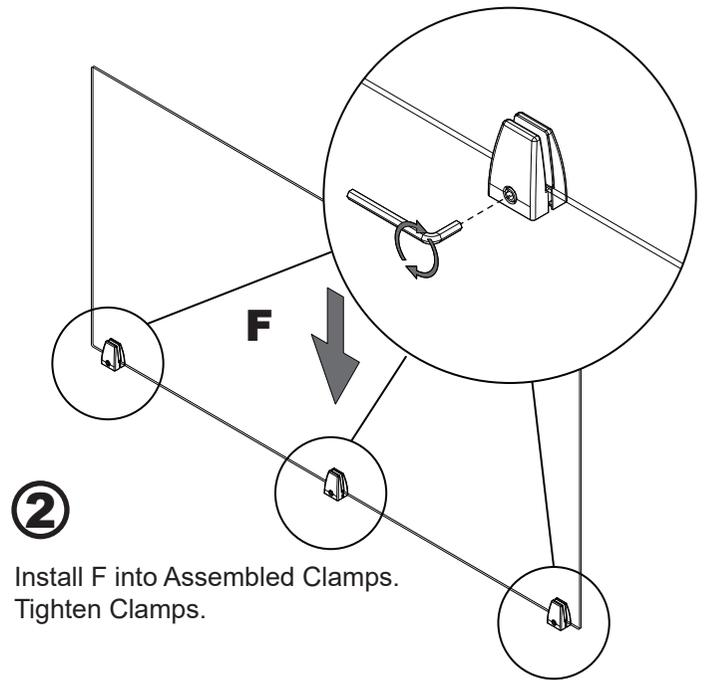
**2** Install F into Assembled Clamps.
