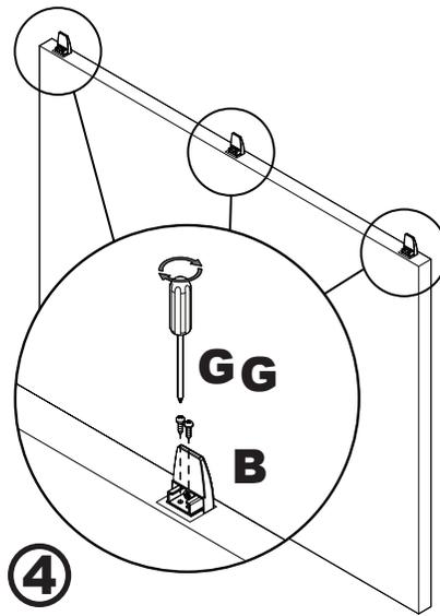
**4** Remove and Disassemble the Panel Assembly. Place Part B on the Wall in the Outline Location and Secure with Screws G.
