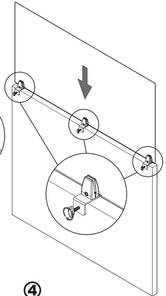
**4** Install Divider Panel onto Wall
