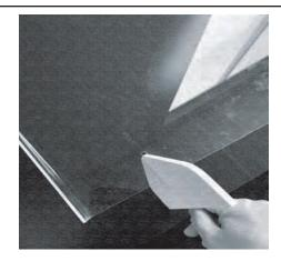
Insert the White Sintra Feet into the pre-cut slots, and press until flush
