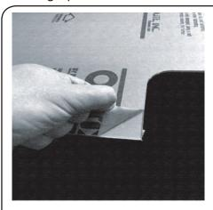
Step 1: Remove the protective covering from the 1/8" plexiglass screen
