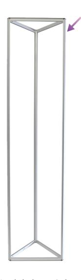
1. Start by lining up a horizontal extrusion with an vertical extrusion. Tighten the lock to secure the connection.
