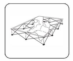
Attach the rest of the graphic by working your way around the frame. Make sure graphic is pulled taut while attaching the velcro.
