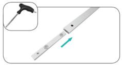
a. Remove screws from Center Connector.
