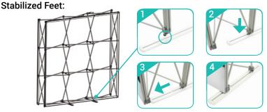
a. From the back, lift frame and insert adjustable feet onto stabilized feet. Then slide stabilized feet toward and insert onto the adjustable feet.
