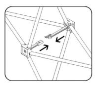
5. Starting at one corner, attach loop on the graphic to hook on the frame.
