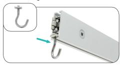
**a.** Eye Hooks: Insert light hooks into the groove in one end of the extrusion.
