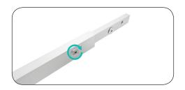
**b.** Tighten screw to lock it into place. Remove the remaining screw from the connector.
