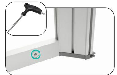
**d.** Connect bottom extrusions together and use torx key to tighten.
