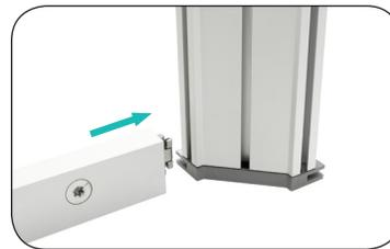
**c.** Connect horizontal extrusion to the bottom of a vertical extrusion, screw facing inward.
