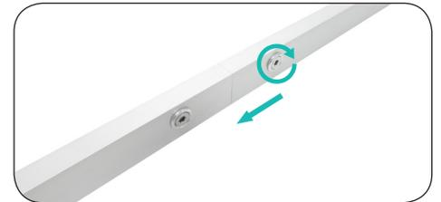
**c.** Then slide the other extrusion onto split connector. Make sure extrusions are flush and tighten the screw to secure connection.
