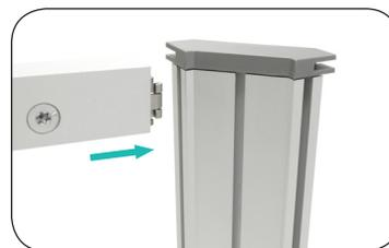
**c.** Connect horizontal extrusion to the top of a vertical extrusion, screw facing inward.
