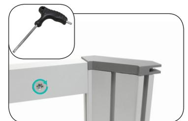
**d.** Connect the top extrusions together and use torx key to tighten.
