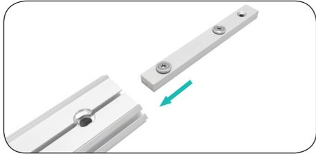
**a.** Remove the screw and insert split connector into one end of the extrusion. Match like colored numbers together. (e.g. 3-3, 4-4).
