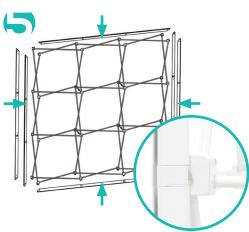
• Attach channel bars to frame. Slide channels bars onto frame, from top to bottom, then secure onto metal peg.
