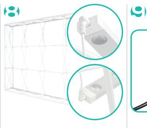
• Plug the Jumper Cords into the top and bottom Edge Lights together.
