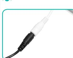
Connect the Jumper Cord to the Transformer using the barrel connectors.
