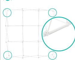
• Connect the top and bottom End Caps on each side of the frame.
