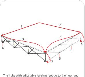
The hubs with adjustable leveling feet go to the floor and are the bottom end of the graphic artwork.
