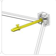
Attach the male arm by popping it into the hub. Fasten the screw through the steel plate hole and the velcro webbing tapping into the female arm.
