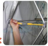
Do not use the yellow locking arms to lift the frame. ALWAYS lift by the frame.
