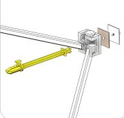
To detach the male arm, remove the screw, steel plate and velcro webbing. Pull the arm off the hub.
