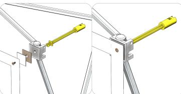
To detach the female arm, remove the screw, steel plate and velcro webbing. Pull the arm off the hub.
