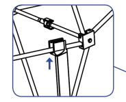
A. Slide top brackets onto X bars on frame.
