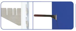
**B.** Check the back side of the frame and make sure the Metal Brackets are hook onto the slots. Insert the Metal Bracket into the pre-cut slot of the graphic and is hook onto the Side Shelf Bracket slot.
