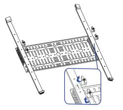
**C.** Attach support struts with the supplied wing nuts.
