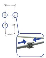
**C.** Close frame by pushing the outside of the frame until male and female ends connect.
