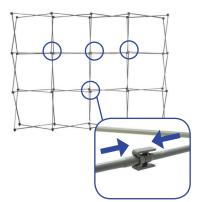
C. Close frame by pushing the outside of the frame until male and female ends connect.
