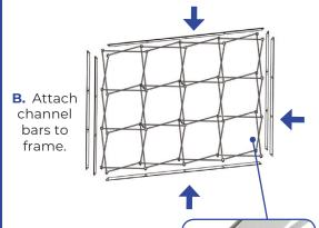
**C.** Slide channels bars onto frame, from top to bottom, then secure onto metal peg.
