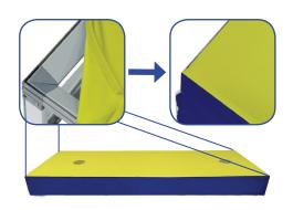
A. In each corner, insert the silicone edge beading into the groove.
