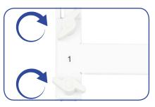
C. Then insert the screw knobs to tighten and secure.
