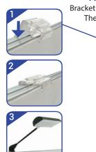
A. Snap the LED Light Bracket on top of the frame. Then slide the LED Light onto the bracket.
