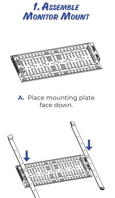
B. Place support struts in desired location on mount.
