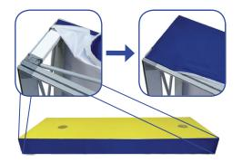
**B.** Install the end cap graphics on each side of the frame. Then insert the remainder of the beading.
