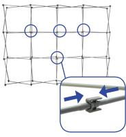
**c.** Close frame by pushing the outside of the frame until male and female ends connect.
