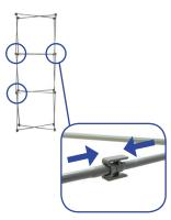
**c.** Close frame by pushing the outside of the frame until male and female ends connect.
