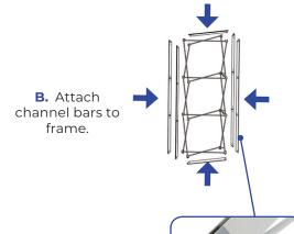
**C.** Slide channels bars onto frame, from top to bottom, then secure onto metal peg.
