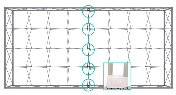
Since the veritcal channel bars will create shadows on the graphics they are not used with 1pc graphics. An alternate method to secure frames without using the Channel Bars + LLW-SCON is using the included velcro straps to connect them. Loop the straps around the X-Rods on the front and back of each frame and secure tightly to secure frames. Reference image above for velcro strap
