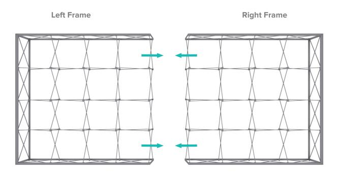
Place the (2) 4x4 frames side by side and connect X-rods with supplied zip ties
