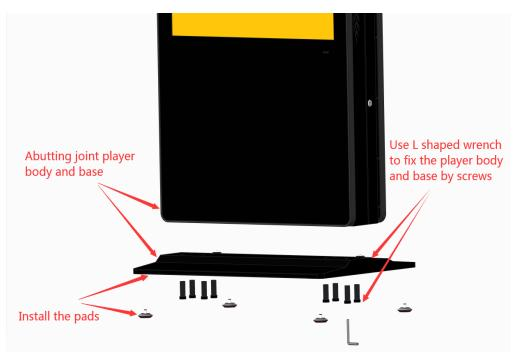
Step 3: Install the pads on all 4 corners and then connect the power cable (back side of player) and power on the player.
