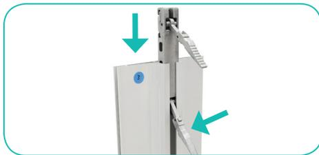
a. Insert tool-free straight connector halfway into top of vertical extrusion. Then press down latch to lock into place.
