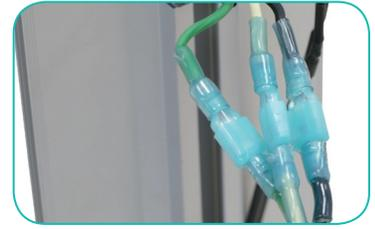
b. Connect and match green, white, and black wiring from transformer to power switch.
