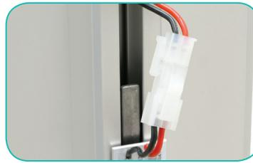
a. Now check light strip connections. Put male and female connectors together around entire frame.
