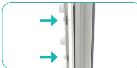
b. Position light strip into inside groove of frame.
