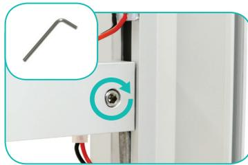
b. Tighten support strut at each end with 4mm allen wrench.
