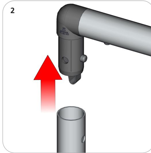
Second, disconnect the snap button connectors at the top of the display wall frame. Continue to remove the entire horizontal row of tubes.
