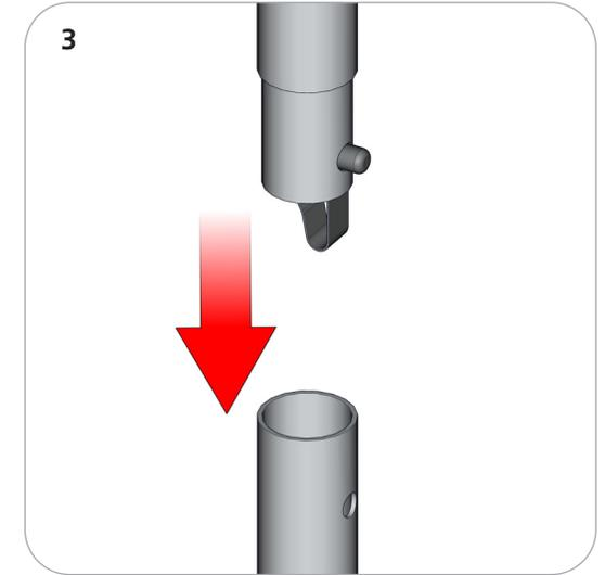
Third, take the male end of the spreader tube and snap it in place of the back wall snap button connectors.
