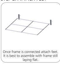
Use provided allen key, secure feet to bottom of frame by screwing bolt.
