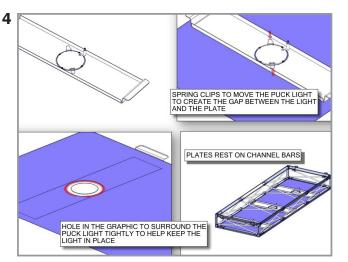
The lighting plates are easily installed. The Plates simply rest on the lower channel bars. For the lighting option you will have a lower graphic with holes. The plates have spring clips which will allow you to adjust the puck light. You will place the circular edges of the graphic cut out along the rim of the light and snap the clip down that way the graphic will sit between the edge of the light and the plate. This will keep your lights in place.
