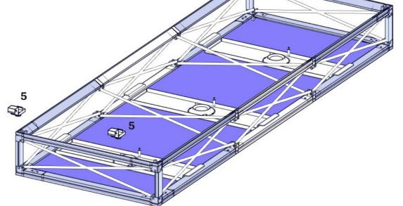
To attach the Bridge connector, simply turn the knob to tighten the end of the connector around the channel bar.
