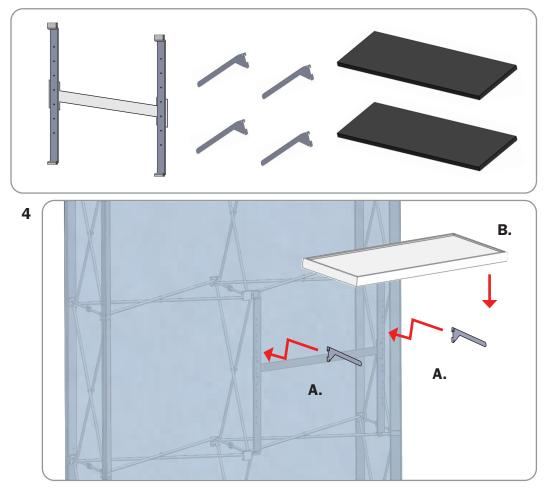
A. After applying the backwall graphic, attach the shelves by placing two arms at the desired height on both brackets.
