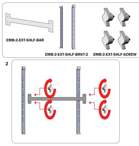
Assemble the mounting hardware by attaching the bar to the brackets - align the holes and use the included screws.
