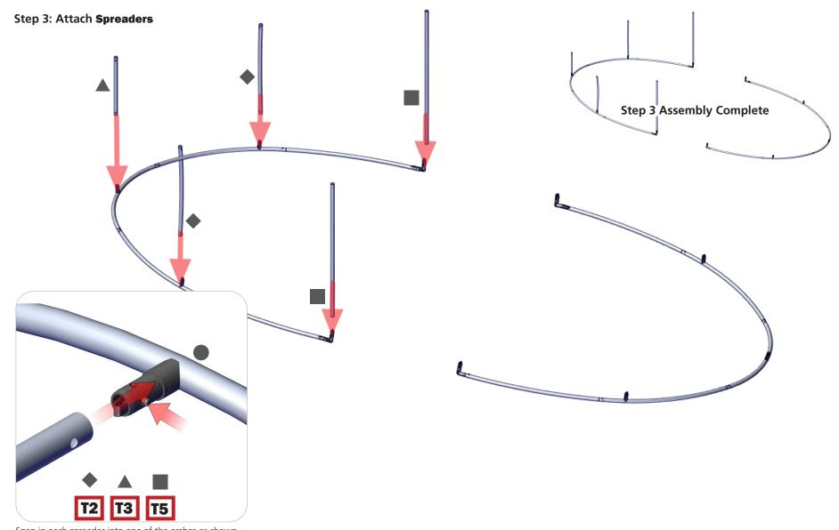
Snap in each spreader into one of the arches as shown above. Refer to to location on page 2. Attaching the 1-way spreader connector into the tubes is easy - simply press the prong in and slide into the tube. With the tube on, make sure the prong comes out all the way through the tube hole. You may have to twist the plastic connector to help align the prong with the tube hole.
