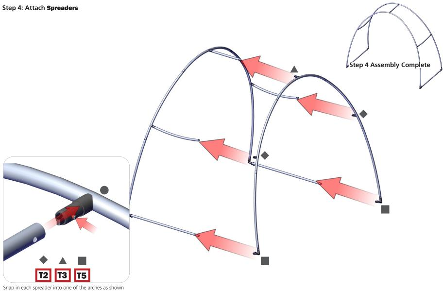
Snap in each spreader into one of the arches as shown above. Refer to to location on page 2. Attaching the 1-way spreader connector into the tubes is easy - simply press the prong in and slide into the tube. With the tube on, make sure the prong comes out all the way through the tube hole. You may have to twist the plastic connector to help align the prong with the tube hole.
