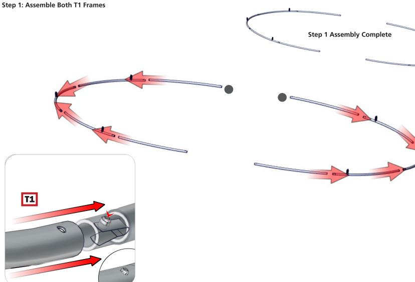
locate the snap button on the connector or swage tube. Locate the hole on the corresponding tube. Press the snap button with your thumb and slide the tube and connector together so that the snap button snaps fully into the lock hole. To disassemble, press the snap button and pull apart.
