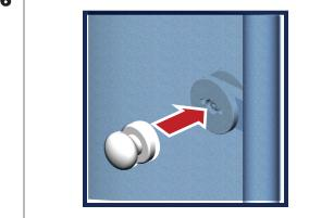
Attach the magnetic door knob to the steel plate attached to the frame. Repeat for both sides.
