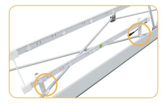
**c.** Hang ladder lights in each section of the frame until reaching the bottom of the frame.
