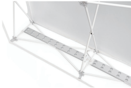
4. Clip edge lights to bottom X rods & connect Y-cables to lights & transformer
