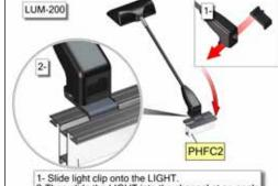
1- Slide light clip onto the LIGHT. 2-Then slide the LIGHT into the channel at an angle and then gently lower down.
